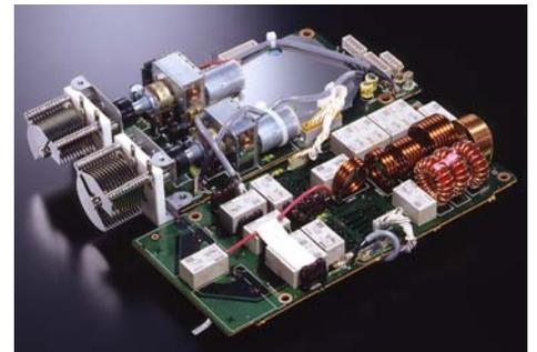
100-Watt Automatic Antenna Tuner
