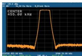
10-pole Collins® Mechanical SSB Filter Passband Response
