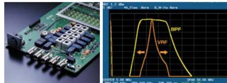
VRF Features Large, High-Q Coils and High-Quality Relays VRF Typical Bandpass Response (3.5 MHz)
